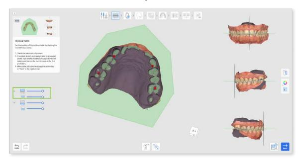
If realignment is necessary, click the "Detach Data" tool at the bottom and manually align data by setting 4 parallel points on the maxilla. As shown below, two are on the distobuccal cusps of the first molars, and two are on the buccal cusps of the first premolars.
