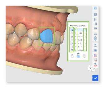
Tooth movement can be performed by the tooth crown, center of resistance, or root apex. Select desired in the Movement Controls widget.
