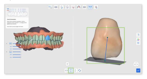
③ To edit the degree of inclination or torque from the occlusal table, click "Inclination (Torque)." Then, choose a tooth and start adjusting by dragging the control points.
