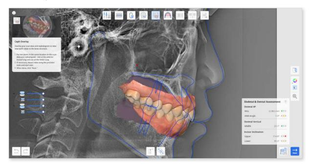
① Check the automatic overlay results. If adjustments are necessary, detach the data from the cephalogram using the "Detach Data" option at the bottom.
