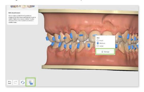
To add a new attachment, click on a tooth. Attachments are available in four shapes: horizontal, vertical, cross, and L-shape.
