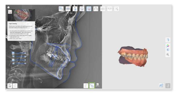
② To manually realign, place two points at the same spot on both the scan data and cephalogram: one at the tip of the front incisor and one at the molar cusp, as shown below.
