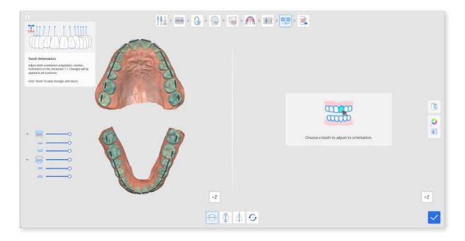
① Click on any desired tooth to start adjusting its orientation; by default, the "Rotation" tool is activated first.
