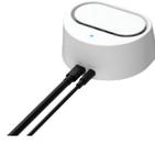
When the i700 wireless is turned on, it will automatically try to pair with the wireless hub. Both the i700 wireless handpiece and wireless hub must be powered and placed in a range of each other to pair. When pairing is in progress, the LED on top of the i700 wireless handpiece flashes. When pairing is complete, the LED lights up. You can start scanning when the pairing is complete.
