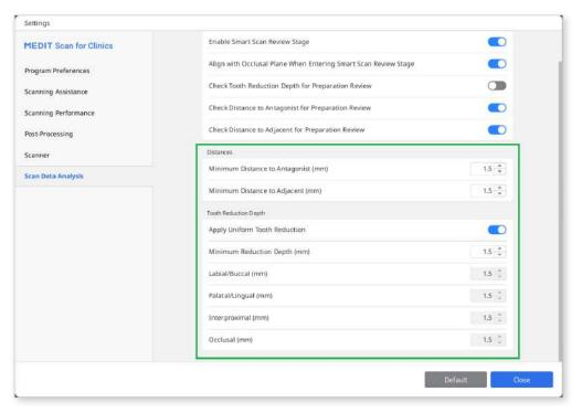
The settings dialog allows users to enter minimum values for distance to the antagonist, distance to the adjacent, and tooth reduction depth to help them establish tooth preparation criteria for treatment and prosthetic fabrication.
