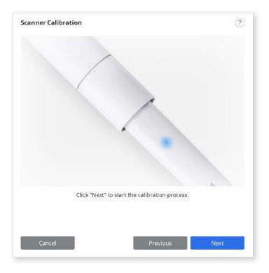
After completing data acquisition at the starting position, turn the calibration tool to the next position according to on-screen instructions.
