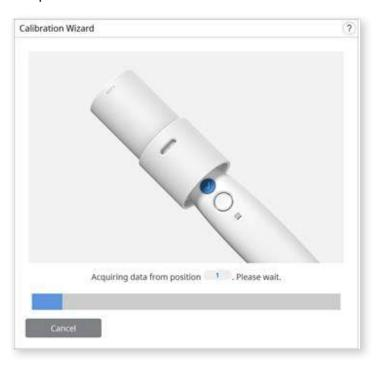
After completing data acquisition at position 1, turn the dial to the next position according to on-screen instructions.
