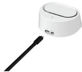
③ Connecting the power cord to the adapter automatically powers the wireless hub.
